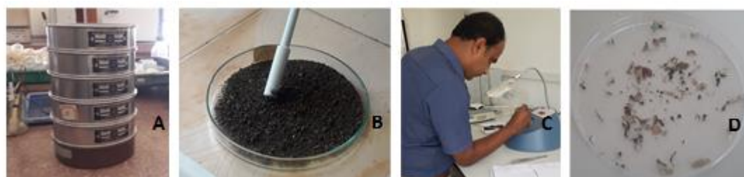
Figure 2: Manual separation of microplastic (A- Sieve set, B-Magnetic separation, C-Manual pick up of microplastic, D-0.5mm to 5mm size separated microplastic)
